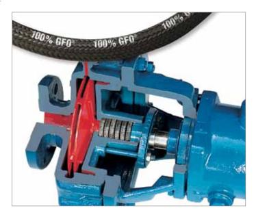
thermal conductivity keep it cool-running even after extended periods of continuous operation at shaft speeds to 4,300 fpm (21.8 m/s). Easy to install and remove, this packing is temperature and chemically tolerant over a wide range of conditions.
